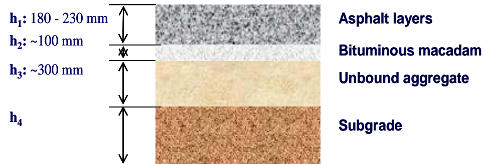
Pavement structure
